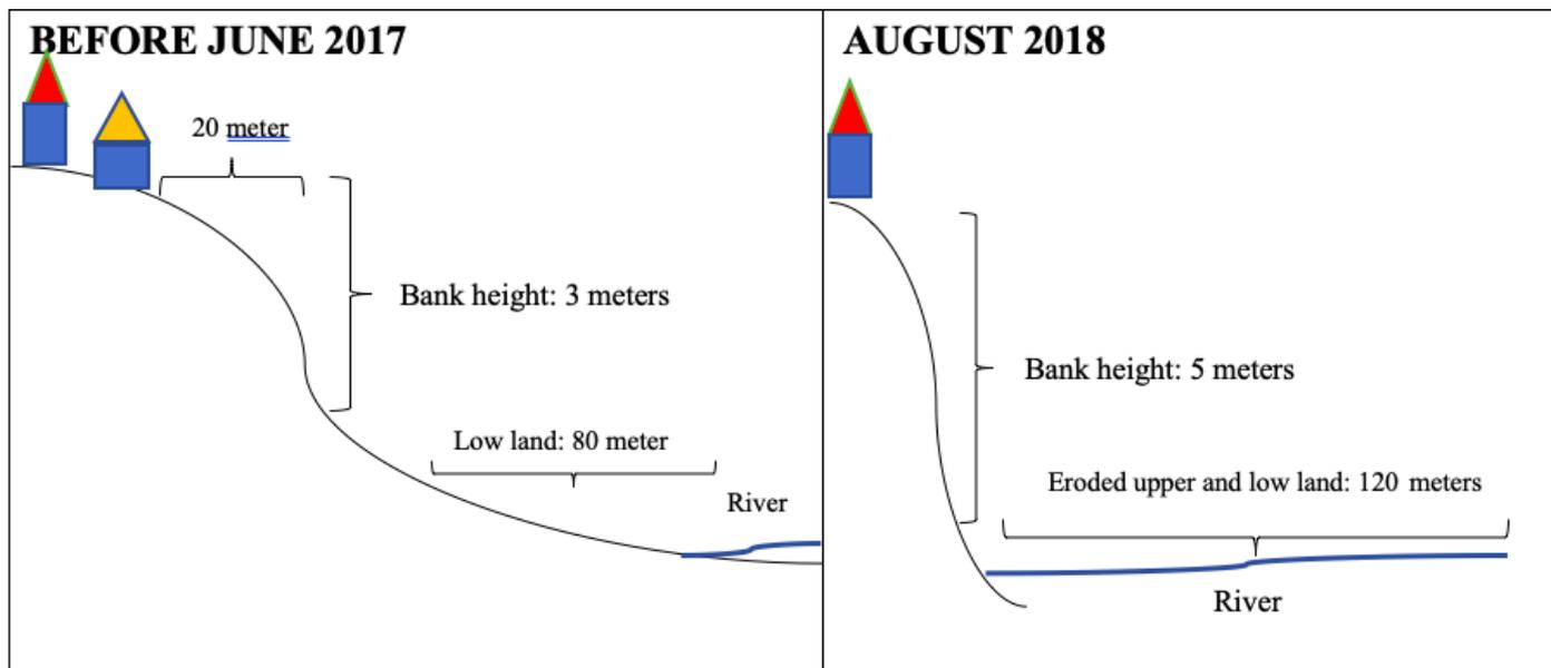
This study also highlights the massive erosion that occurred at Kg. Pasir Parit as a result of the existence of a river barrier. The barrier is made of an iron rod and is around 6 metres tall (KADA, 2018). KADA built this barrier to divert water flow to their pump house, enabling them to provide water for farming and agriculture (Figure 2).
