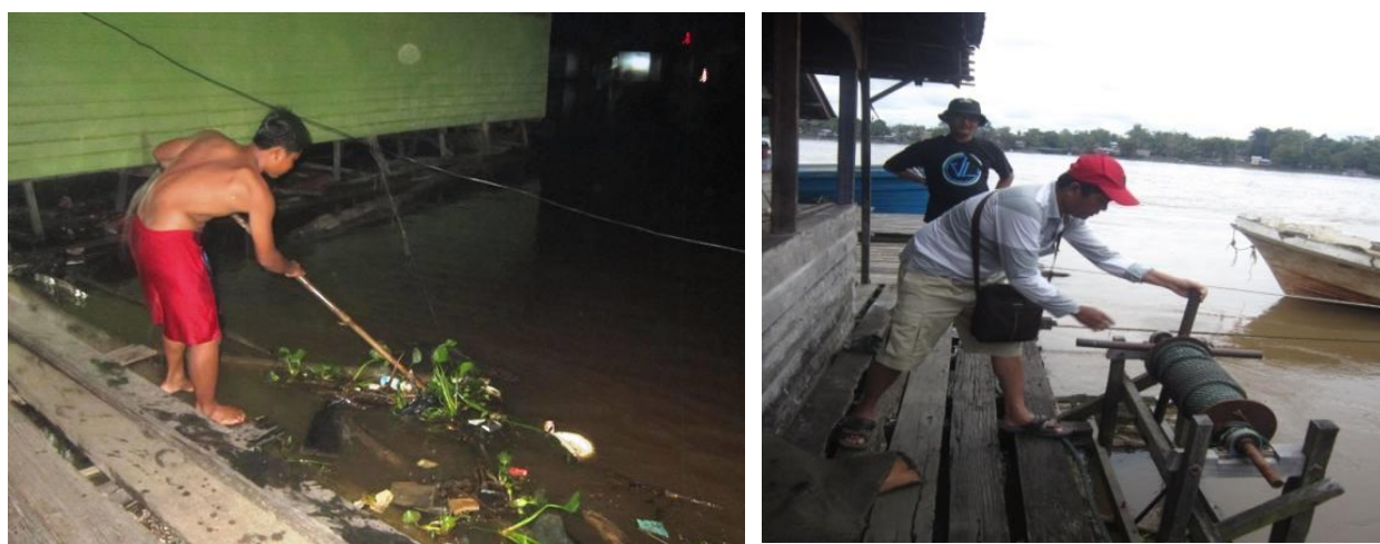
Figure 7 (left). Cleaning stuck trash during night-shift; Figure 8 (right). Mechanical reel to adjust lanting position with fluctuating water level (Photos: Albertus Imas, 2018)
