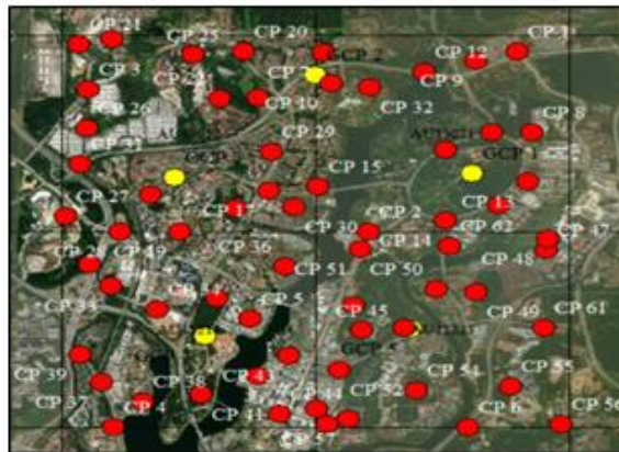
Figure 4. Location of GCP (yellow points) and CPs (red points) over the study area
