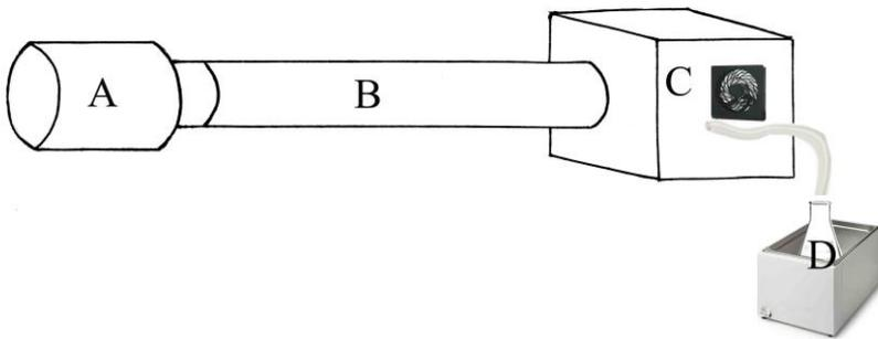
Figure 1. (A) release chamber; (B) flight tunnel; (C) trap and dispersion chamber; (D) lure chamber.
